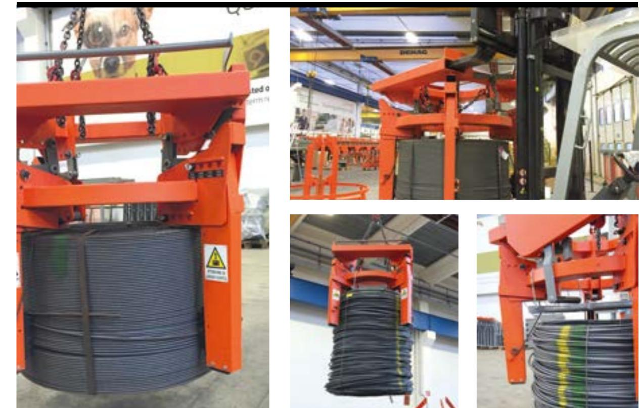
Internal Spider is a safe clamp with small dimensions which, thanks to its innovative shape allows the hooking of the rewinded coils from the inside.
