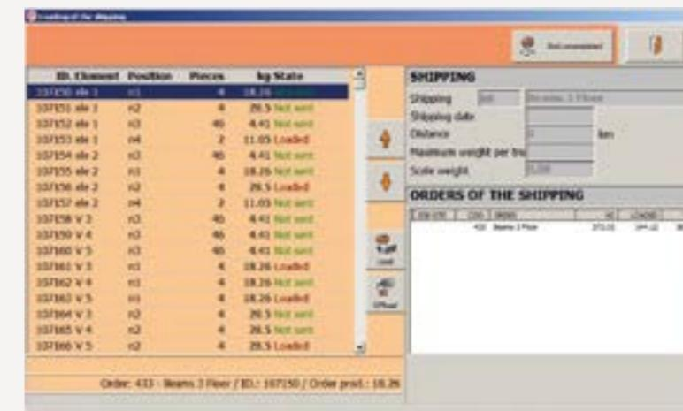
It allows a real time control of the material loaded into the trucks, it checks the conformity of the cargo and it prints the appropriate transport document.
