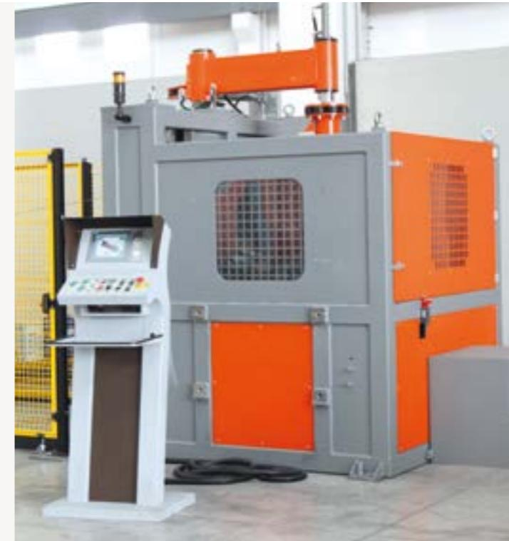
Vertical spooler, allows collecting the wire on the spooler. It is provided with wire guide at variable pitch. Max weight of the spooler: BV 3000 kg, BVC 3000/5000 kg.
