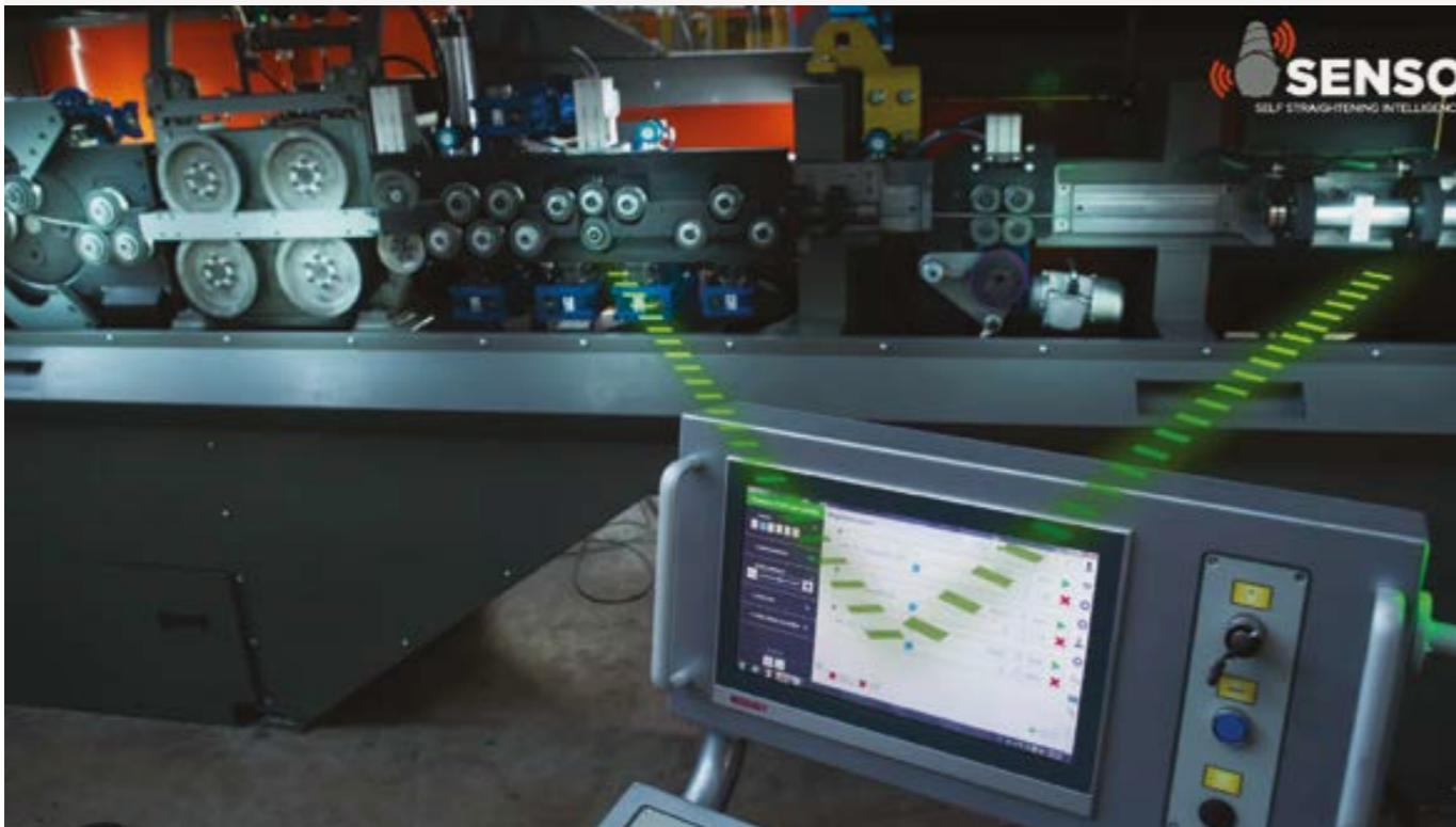
The sensors detect the curvature in the wire that is being processed and interact with the machine's software, exactly as an expert operator would do, modifying the settings on the straightening system. The result is stunning: the bars are always straightened perfectly and the speed is very high.
