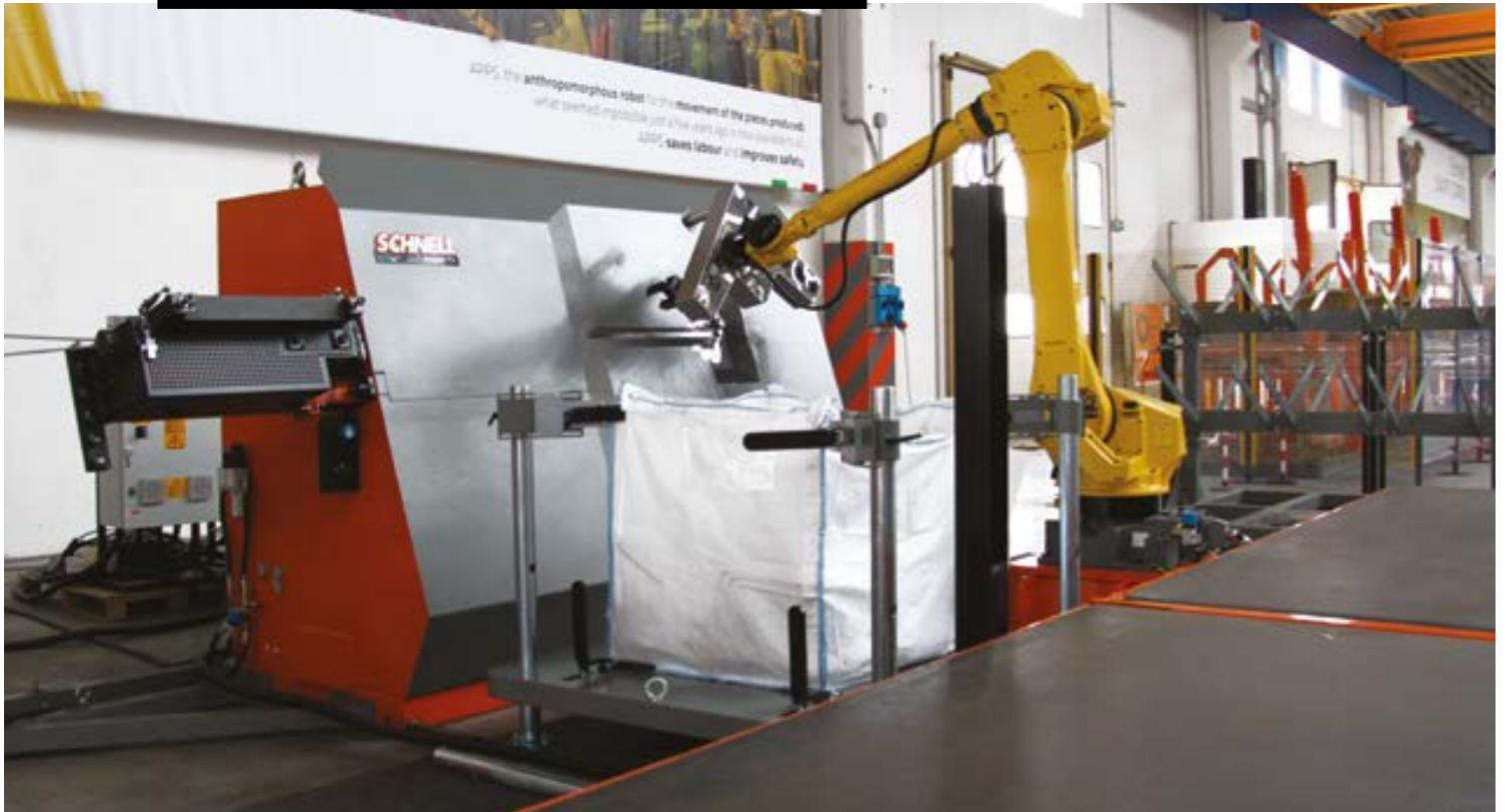
**APPS saves labour and improves safety.** Automatic Robot able to pick straight bars and stirrups of variable shape and size directly from the stirrup bender and to pack them in predefined zones within a safe working area.
