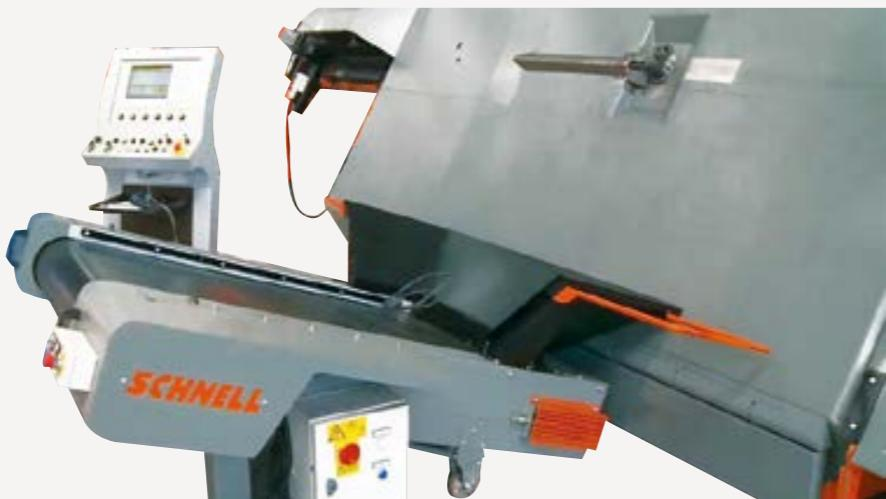
Conveyor for the collection and the transport of the stirrups produced by the stirrup machine.
