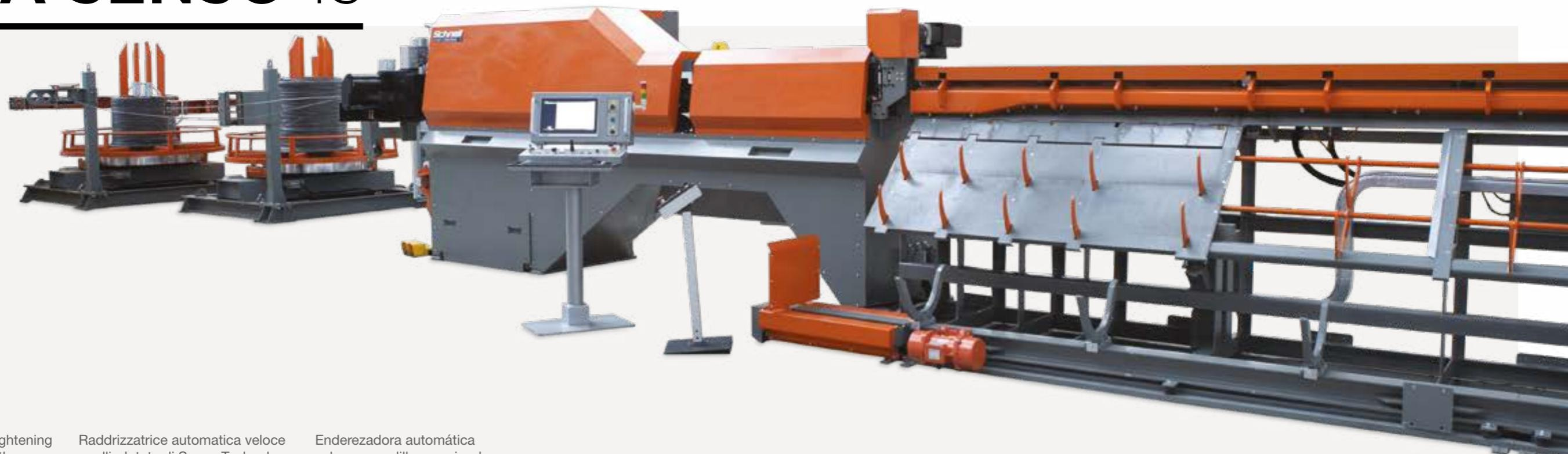
Fast automatic wire straightening machine, with rollers, for the production of cut-to-size wires up to Ø 13 mm (#4), equipped with Senso Technology.
