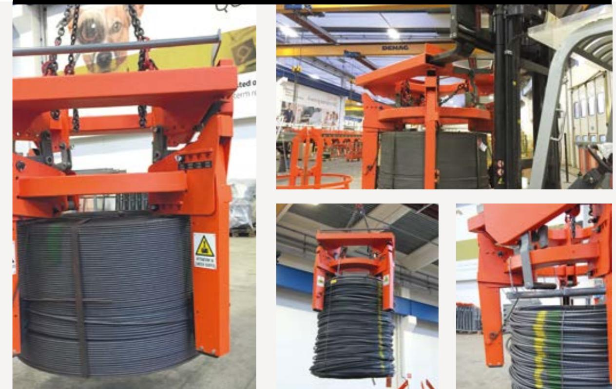
Coil Spider is a safe and small lifting device that, due to its up-to-date features, can hook from the outside rolled and drawn coils.
