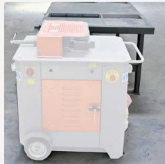
12. **BLF/3** Bending bench equipped with idle rolls and working platform.
