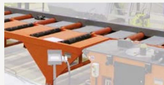
13. **B12 MFC** Bending Bench with 2 roller tracks: 1 track with rubber-lined motorized rollers, and 1 roller track with idle rolls.
