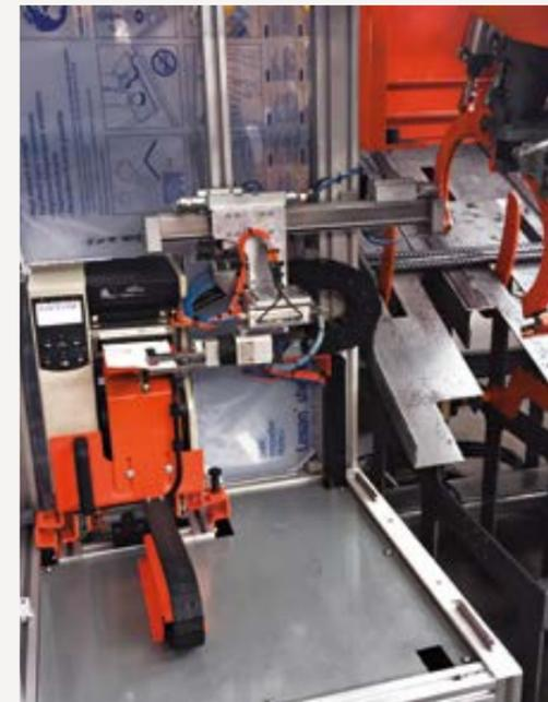
**SMART TAG** automatically attaches the tags to the bundles during the tying phase.
