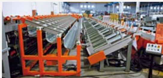
4. **POCKET** Soundproofed cradle storage optimiser. it can be loaded and unloaded without any priority or sequence restriction. is not required.
