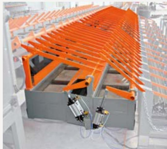
9. **T** Storage optimisers. Allows completion and lengthwise transfer of bundles of bars requiring subsequent bending.
