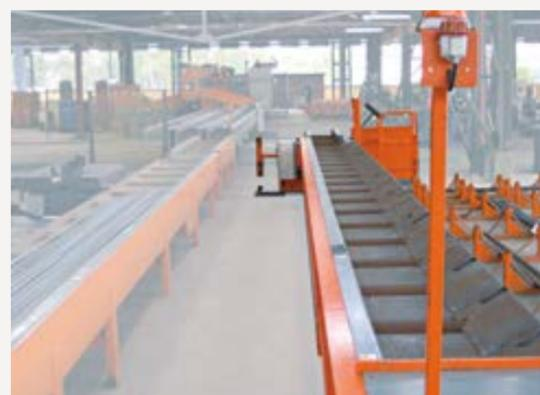
10. **CC** Mobile commissioning carriage. To unload the cut bars onto the floor classifying them in specific deposits.
