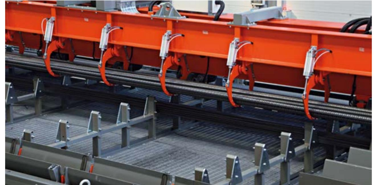
**The automatic feeder Mega Genius** is our latest novelty. It takes, counts and moves the bars for shear-line feeding in a completely automatic way.
