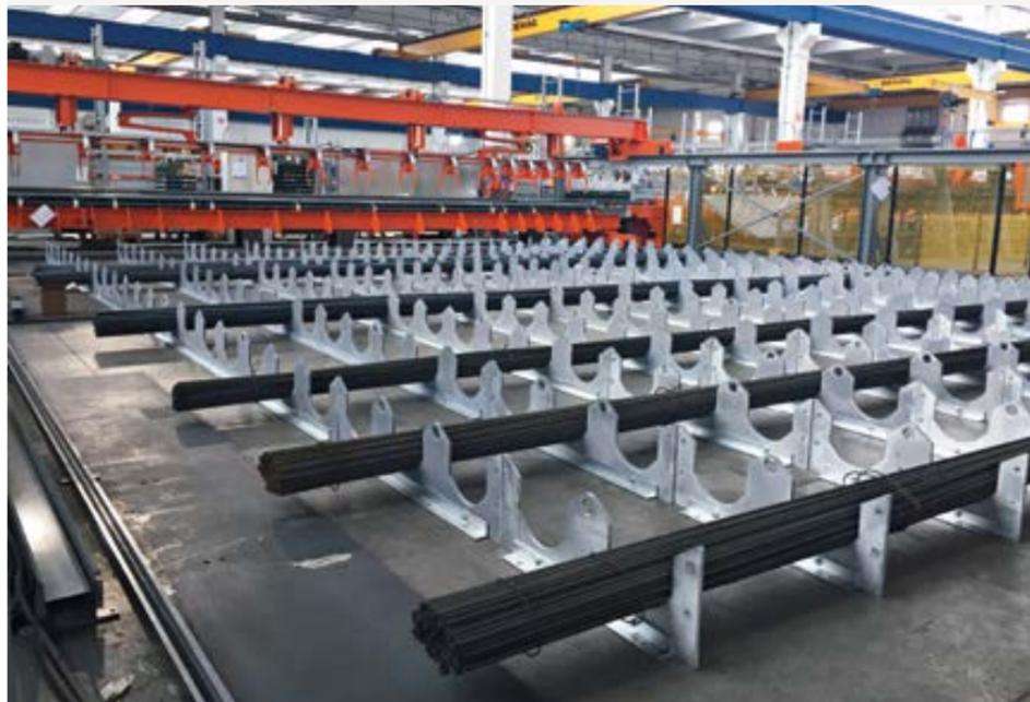
**GROUND BUFFER** is an innovative system to deposit, storage, taking bundles of bars, labelled and tied, coming from the Shear Lines o Reta line.
