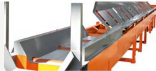
11. **VRP** Distribution tracks. They allow storing cut bars and act as storage unit for subsequent working operations.
