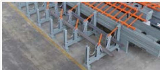
3. **RACK** The rack allows collecting the cut bars and making them up into bundles when further processing is not required.
