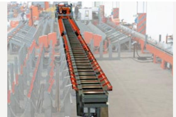
15. **VS** Unloading track. It has the function to receive the bars from measuring and transfer track (VMT) aligning it and to unload the bars on the storage sections.
