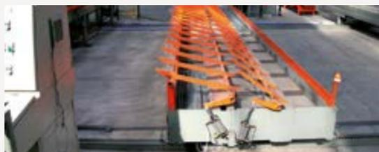
6. **CPO** Mobile optimizing roller carriage. For storing and transferring bundles of bars cut to size towards subsequent machining operations.
