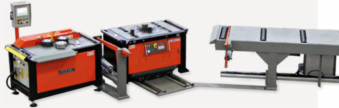
IPC 40 is the plant for the production of radius bars with bends in a single, automatic process. It is composed of the radius machine CER 40, the bidirectional-bending machine P 45 PRO and has an unloading system for the completed bars.
