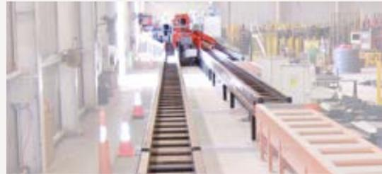
8. **PT** Roller conveyor. Allows lengthwise transfer of bundles of bars.
