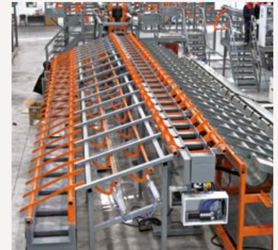
16. **SDS** Pneumatic storage slide. Slide with 2 pneumatic arms for bars collection, able to transfer the bars to the close bending bench or bending robot.
