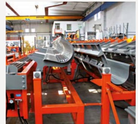
17. **Lifting buffer** It receives the bars from the Shearline pockets and lifts them onto the roller track of the bending robot.
